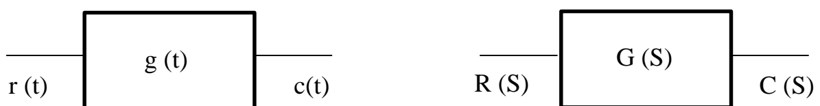
Figure 1 : The left side is a system in time domain – The right side is the system in frequency domain.
