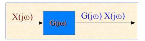
That is, making  $S = 0 + j\omega$  in the transfer function G(s), one obtain  $G(j\omega)$
