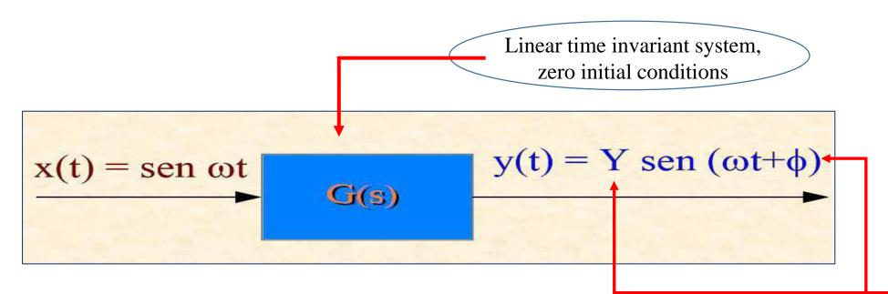
The output y(t) will have the same *frequency* of the input x(t), but, the amplitude Y and the phase angle  $\phi$ , will be, in general, *different*.
