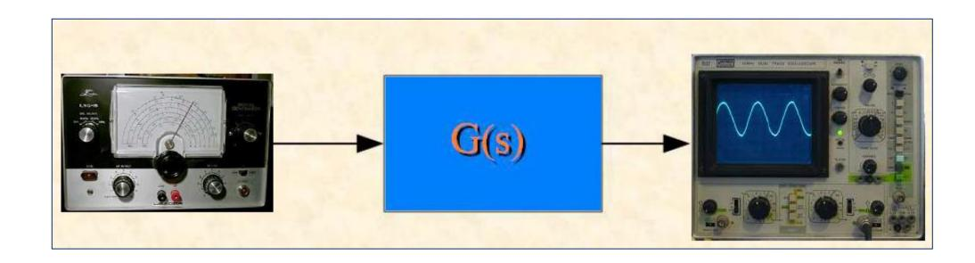
Therefore, the analysis of complicated systems can be done through tests of *frequency response* without being necessary to determine the *roots* of the characteristic equation (i.e., the *poles* of the *system*)
