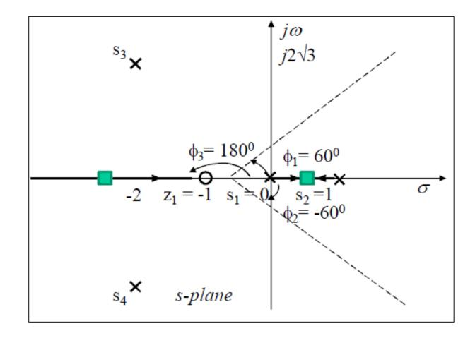
5. Determine the angle of departure (angle of arrival) of the root locus from a complex pole (at a complex zero).
