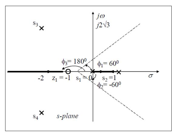
4. Find the breakaway and break-in points: Depending on the characteristic equation P(s).
