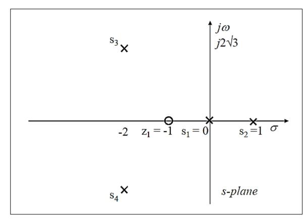
2. Determine the root loci on the real axis: Root loci exist on the real axis between 1 and 0 and between -1 and  $-\infty$ .
