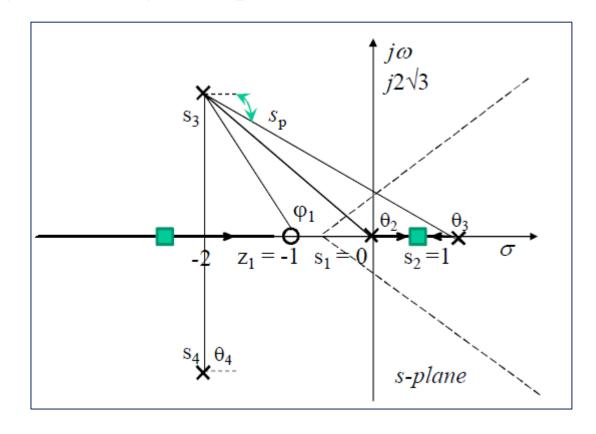
6. Find the points where the root loci may cross the imaginary axis: letting  $s = j\omega$  in the characteristic equation, equating both the real part and the imaginary part to zero, and solving for  $\omega$  and K.
