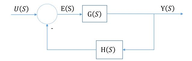
The closed-loop transfer function poles are the roots of the characteristic equation.
