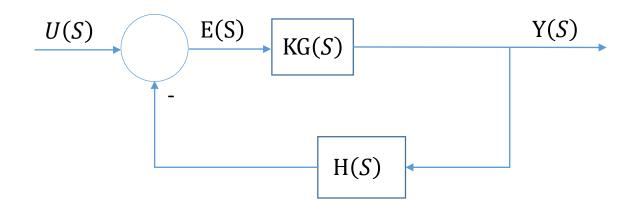
The root locus is the locus of roots of the characteristic equation of the closed loop system as a specific parameter (usually, gain K) is varied from zero to infinity,  $0 \le K \le \infty$  giving the method its name.
