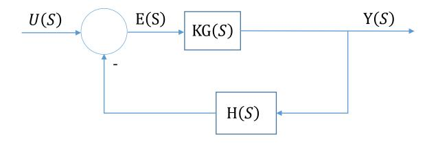
**Angle Condition:**  $\angle KG(S)H(S) = \pm 180^{\circ} (2K + 1), (K = 0,1,2,...)$
