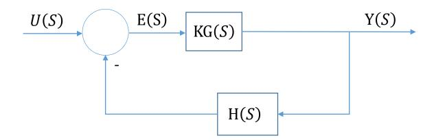
If the system has a variable loop gain, then the location of the closed-loop poles depends on the value of the loop gain chosen. It is important, therefore, that the designer know how the closed-loop poles move in the *s* plane as the loop gain is varied.
