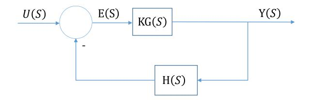
A simple method for finding the roots of the characteristic equation has been developed by Prof. W. R. Evans in 1948 and used extensively in control engineering. This method, called the *root-locus method*, is one in which the roots of the characteristic equation are plotted in complex  $S = \sigma \pm j\omega$  plane for all values of a system parameter.
